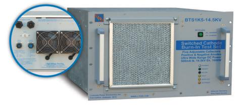
The CPE Burn-In Test System (BTS) is a TWT power supply used for production aging, predictive failure analysis, and RF experimentation. The BTS offers high voltage, patented series-stackable resonant converter modules that provide 3 to 5 collector outputs plus a cathode output ranging from 1000V to . 14.5kV at a maximum of 500mA lk and 1000W. Each converter can supply 250V to 4500VDC differential voltage up to a wide load range of 400W per module with 1% voltage and current regulation.
